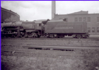
A Pennsylvania locomotive and coal car roll into the maintenance yard. Locomotives had to be pulled from duty about every 100 miles to keep them in good working order.
